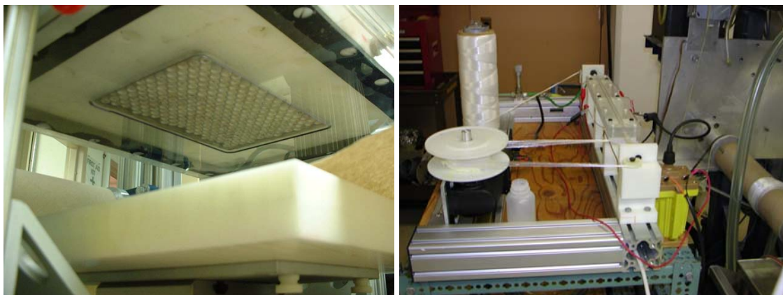
Figure 2. Atmospheric plasma reactors: AER (left) and CP (right).
