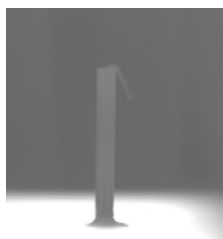
Figure 1. An infrared imprint of a polymerization front experiment. The white bottom surface is a hotplate at 90°C where a glass tube filled with DES is placed to promote the polymerization. The external diameter of the glass tube is 7 mm. At the top of the tube it is observed the cotton cord wet with the initiator that goes from the bottom of the glass tube to the top.
