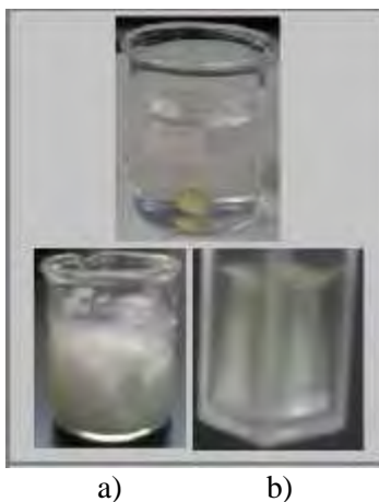
Figure 1. Results sol-gel technique, a) spherical silica powder, using hydroxide and b) silica glass, using nitric acid.
