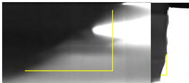
Figure 5. At left, a space-time plot where a polymerization wave starts near the top of the tube. At right, a polymerization front with four cotton cords inside the glass tube, what grants four times the local amount of Luperox 231 with respect to the experiment described in Figure 2. Evidently, the front advances much faster.
